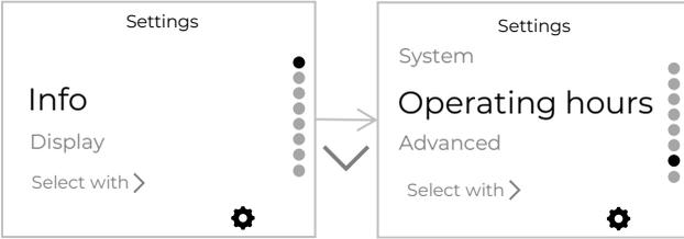
Display of operating hours for the heat pump, electric heater, external heater, primary and secondary ducts, recirculation, and number of defrost cycles.
