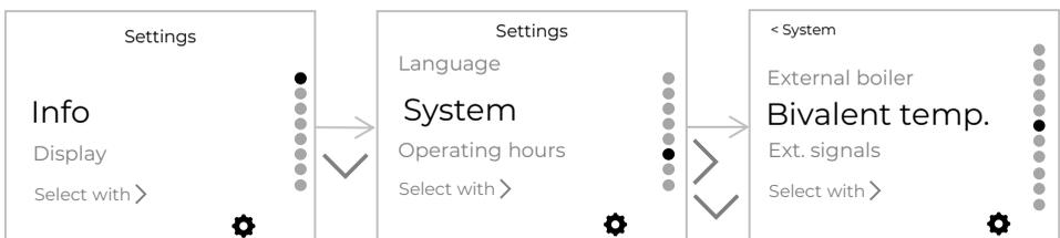
When the inlet air is colder (below 3 °C), the heat pump operates at reduced power. At this point, the selected additional heater (electric heater, oil, gas, or pellets boiler, etc.) can be activated for assistance. Setting the bivalent temperature determines at which temperature this additional heater turns on. When the inlet air temperature rises 3 °C above this value, the additional heater turns off automatically.
