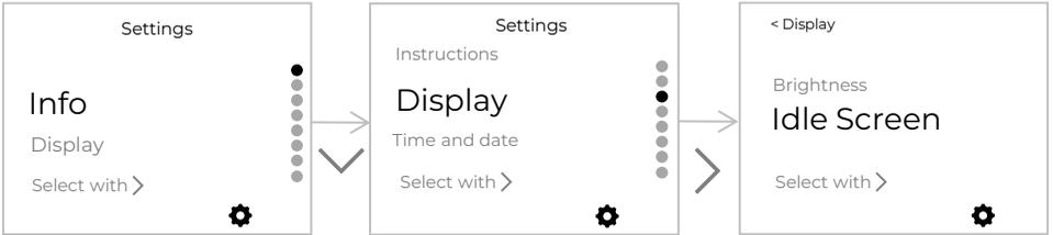
The display switches to sleep mode after 5 minutes of inactivity. In sleep mode, the screen displays one of three options: off (none), time, or temperature.
