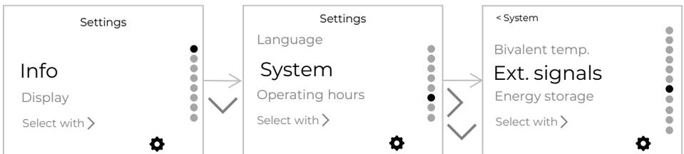
The device control can accept up to 2 customizable external signals. Possible settings are described in the table below.
