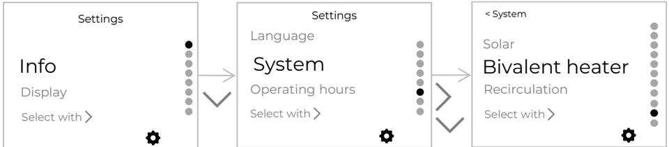
The bivalent or additional heater is used to support the operation of the heat pump. It also activates in the event of a heat pump malfunction.
