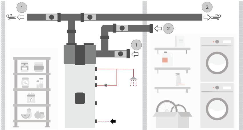
Figure 1: Example of selecting primary and secondary ducts
