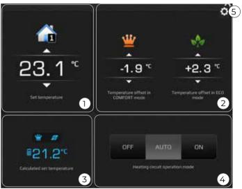
1 Setting the temperature in NORMAL loop mode. The temperature shows the set desired appliance parameter . Use the arrows to change the desired temperature.
